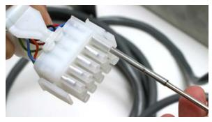
**DO** use a pin pusher to remove the 15-pin plug on the controller cable for routing.
