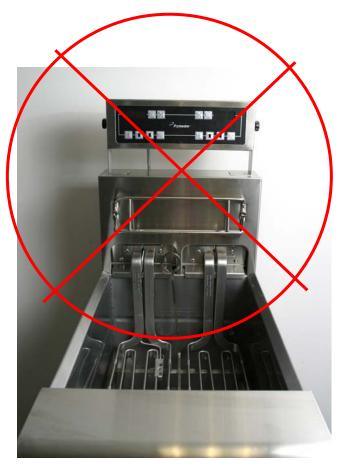
**DON'T** mount the controller on the fryer's tilt housing or on the bulkhead above the fryer's vat
